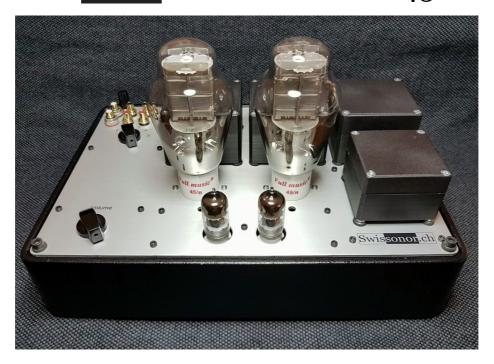
**45SE** = Integrated tube amplifier with type **45** triode in **SE** configuration
